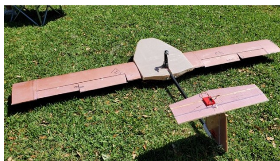
(b) Actual flight test ready SAILR UAS weighing 10.5-lbs
