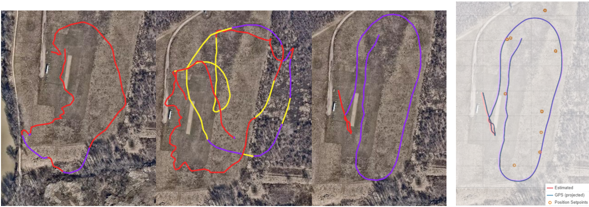
(a) Flight log from three tests (from left: manual, altitude, & mission mode flight)
