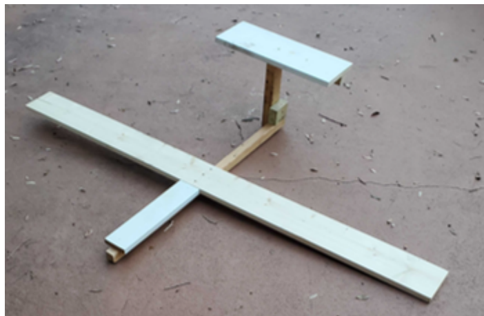
Figure 18: An 8-lb glider made from scrap wood
