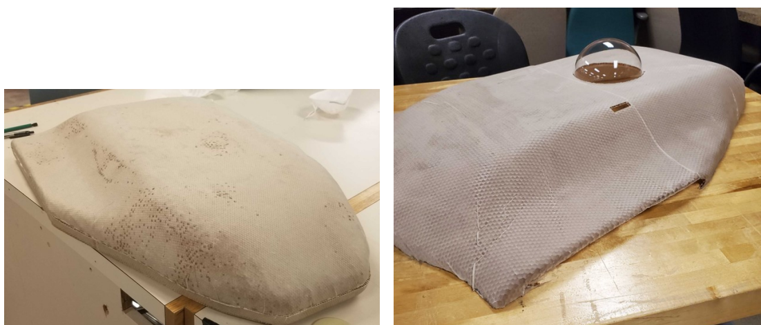
(a) Version 1 of the fuselage with 1/4" Nomex and pour-as-you-go epoxy (b) Version 2 of the fuselage with 1/8" Nomex and premeasured epoxy
