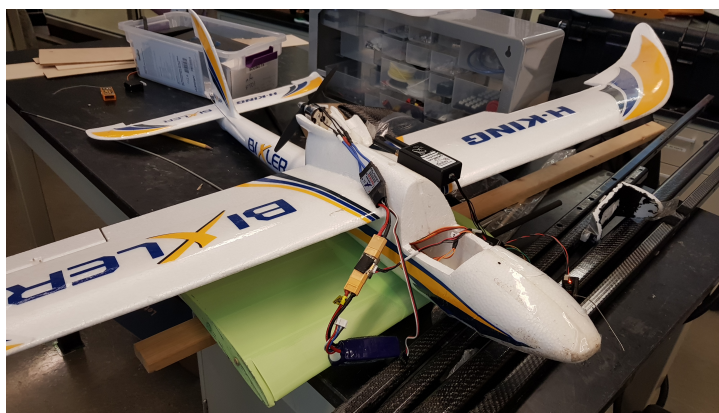
Figure 36: Modified Bixler Trainer Aircraft configured with SAILR avionics
