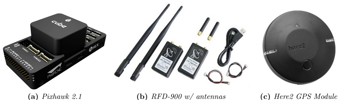
Figure 17: Control system components
