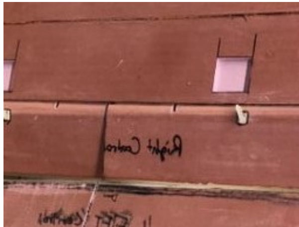
Figure 24: Curvature of the Wing-Aileron Joint
