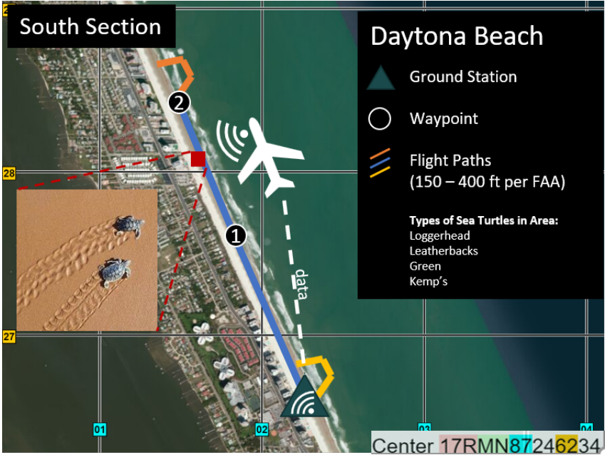
Figure 8: Mission profile applied to the section of Daytona Beach stretching from International Speedway Blvd. to the city limit covered by the Volusia County Sea Turtle Conservancy. Yellow- takeoff & ascend, blue- cruise, orange- descend & land.
