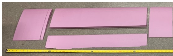
Figure 25: One wing is shown separated into the root and tip sections with the third section, the center, having the control surfaces cut out.
